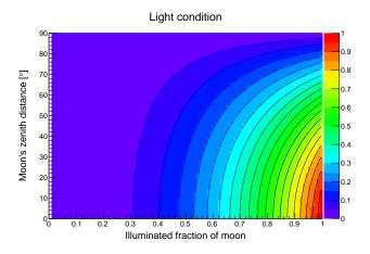
**Figure 1**: Light condition. As color scale, a value describing the background light condition is plotted versus the moon's illuminated fraction and the moon's zenith angle. It is proportional the measured median current in the camera. Each contour level corresponds to a step of 0.05. The values range from new moon condition (0) to the worst possible condition at full moon (1).
