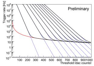
**Figure 2**: Top: Ratescans taken close to zenith at different light conditions between dark night conditions and almost full moon conditions. Bottom: Parametrization for ratescans depending on the measured median current with  $10\mu A/\text{ch}$  spacing. The power-law of the proton spectrum (red) and the background spectra (black).
