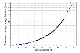
**Figure 4**: Relative worsening of the energy threshold expressed as a ratio versus the zenith angle  $\theta$ . The black points are simulation results for the MAGIC telescope and were taken from [6]. A fit to the data (up to 60° zenith angle) in  $\cos^{\alpha} \theta$  is overlayed as blue line.
