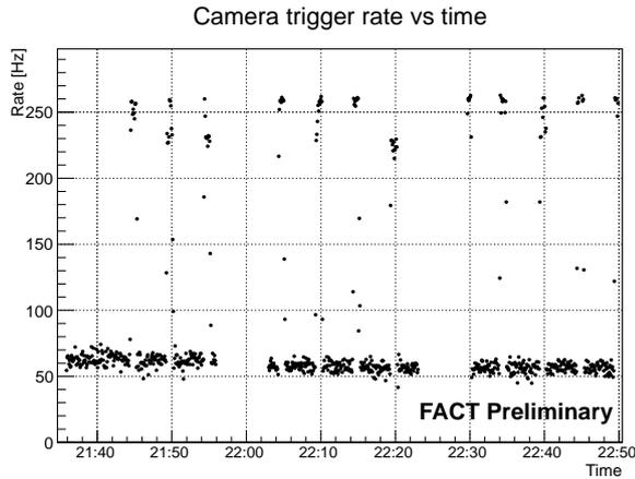
**Figure 1:** FACT readout rate saturates when a Lidar is in the field of view.
