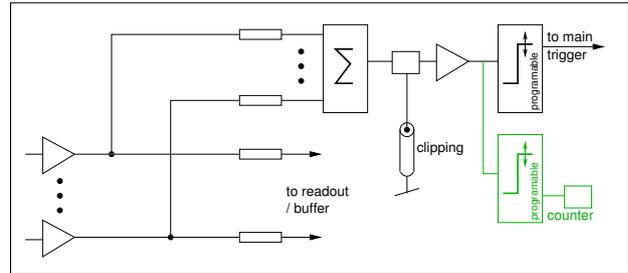
**Figure 9:** Using two independent comparators, rate scans can be done during data-taking.
