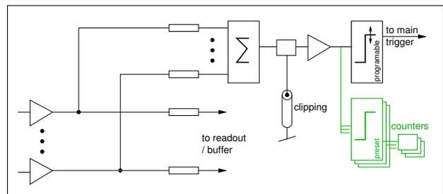
**Figure 10:** Using several comparators, same information can be gained without a scan during data-taking.
